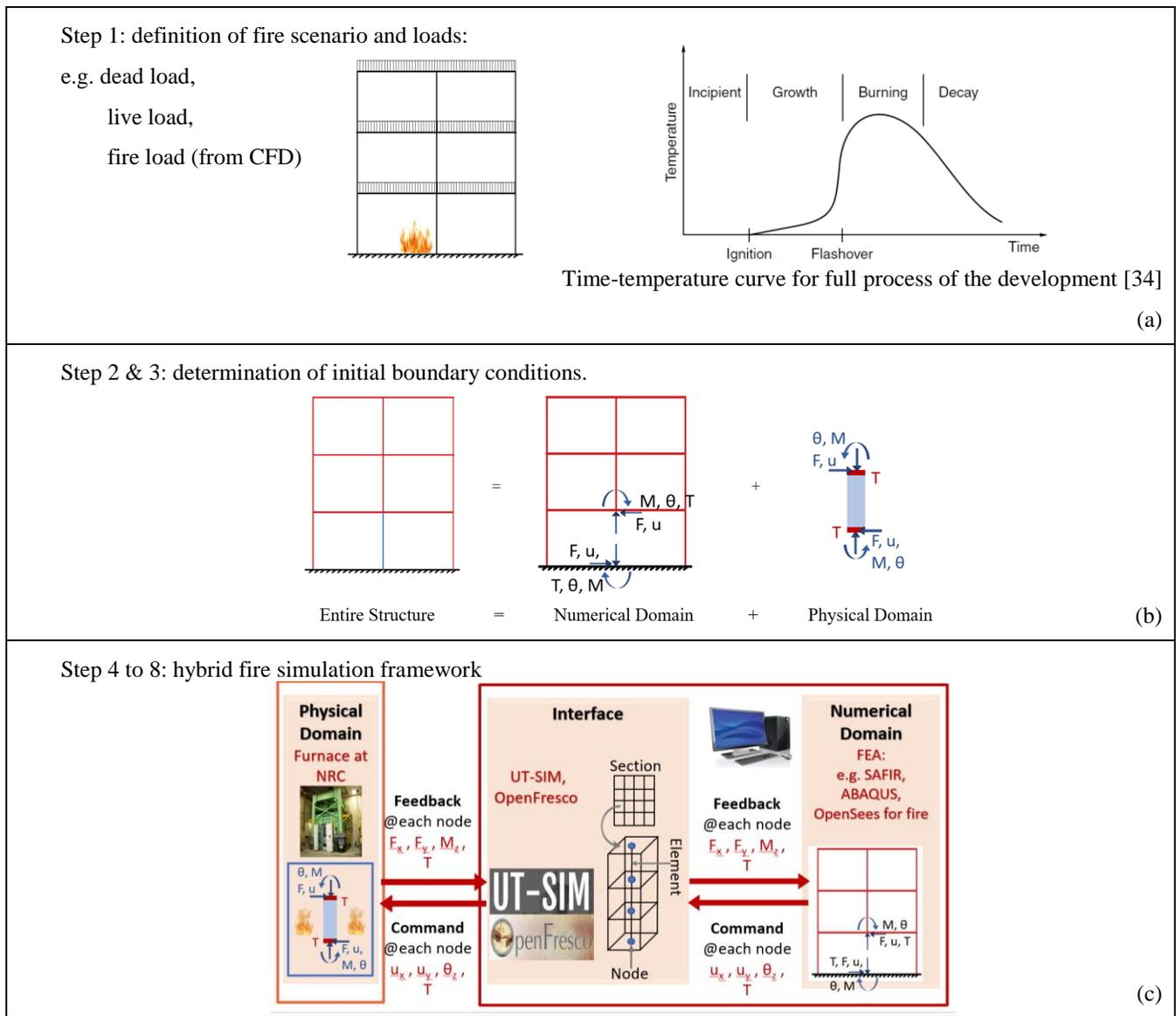
Figure 5. Process of hybrid fire simulation.
