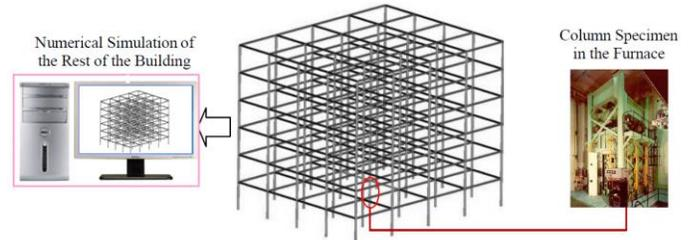
Figure 2. The HFS components for the 6-storey building [17].
